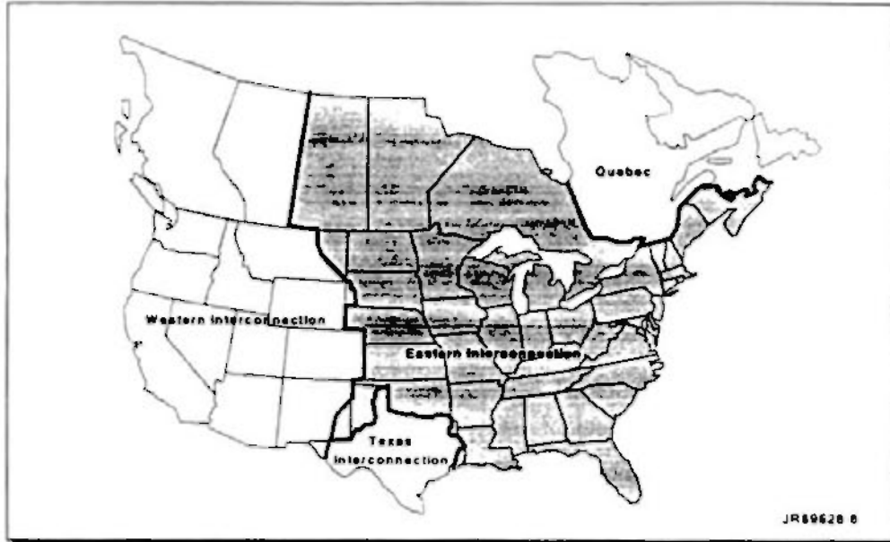
Figure 1: Interconnections of Utility Systems
