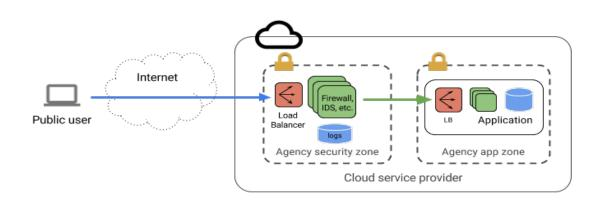
An example diagram showing data-centric security in a cloud provider is shown in **Figure 1**.
