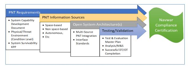
**Figure 1. NAVWAR Compliance Process Components**
