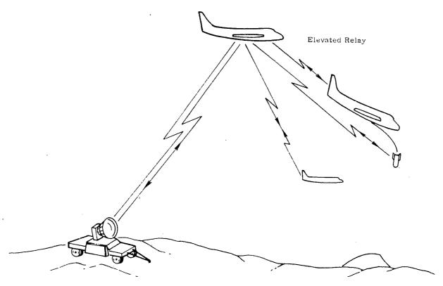
Figure 1. Elevated Relay Operation
