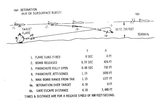
Figure 10. Typical Beckett trajectory diagram
