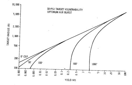
Figure 3. Target radius versus yield required for expected fractional damage  $\geq 0.9$
