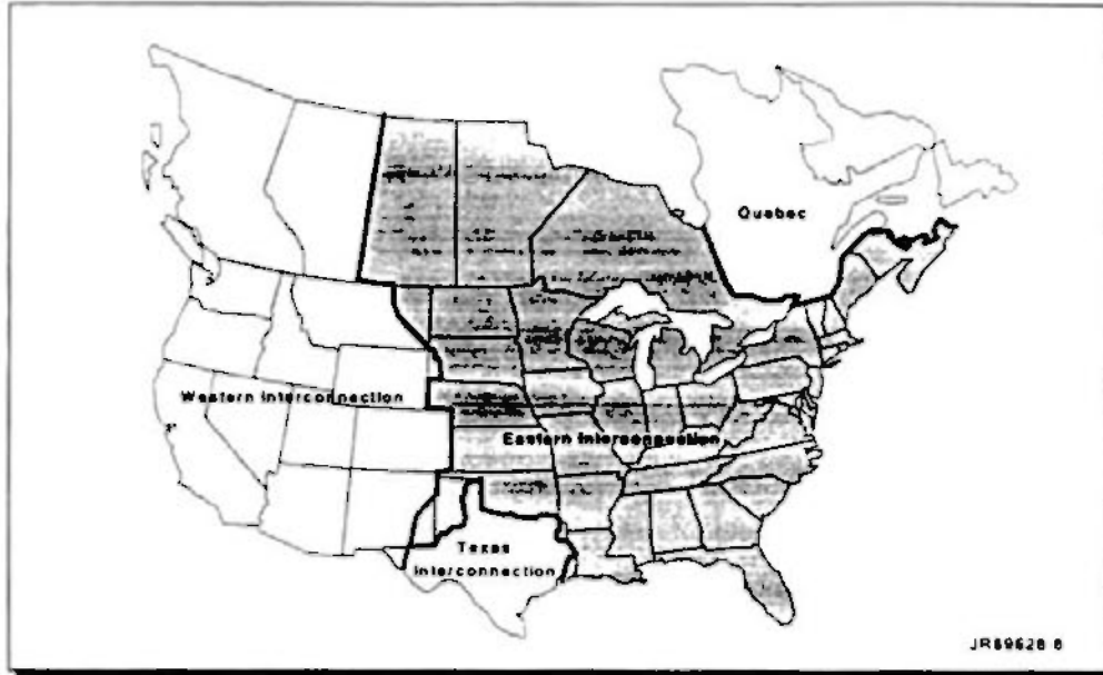
Figure 1: Interconnections of Utility Systems
