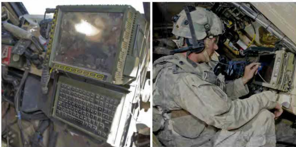
Joint Battle Command – Platform (JBC-P) Joint Version 5 (JV5) Block 2 Display and Keyboard (left) and Commander using JBC-P (right)
