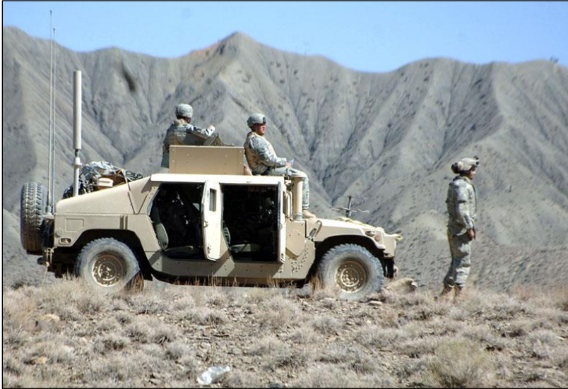
Figure 3. Duke Version 3 Vehicle Mounted CREW system
